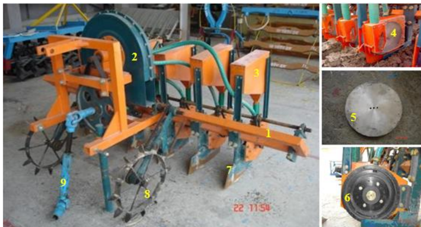
Figure 1. Pneumatic planter during in laboratory evaluation. 1. Frame; 2. Aspirator blower; 3. Seed hopper; 4. Metering unit; 5. Multi groove metering plate; 6. Vacuum retaining plate; 7. Furrow opener; 8. Ground wheel; 9. Cordon shaft.
